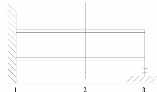
Fig. 7-5. Propped cantilever beam
